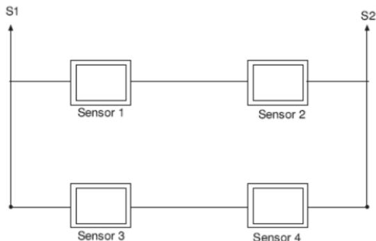
**Fig. 1 – Remote Room Sensor – Parallel Wiring**
