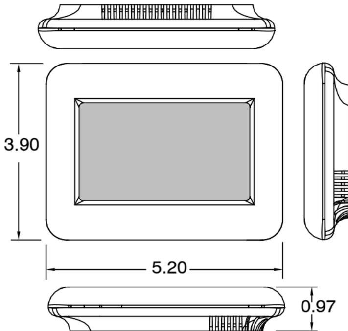
**Fig. 2 – Wall Control Assembly Pieces
