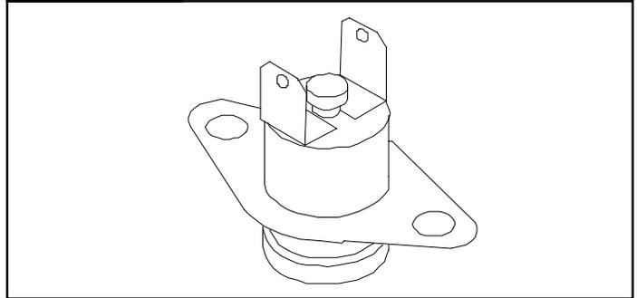
To verify this, the cut-out (opening) point of the switch should be checked (using a thermocouple type thermometer connected to the face of the switch) as follows:
