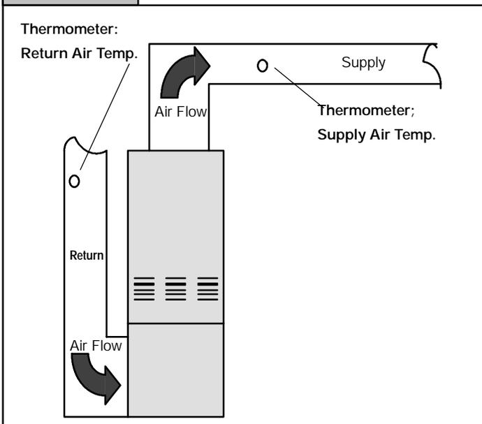
Simply stated, the temperature rise through the furnace is the difference in temperature between the return air, and the supply air.
