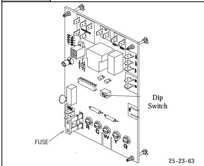
The Honeywell ST9160B Electronic Fan Timer/Furnace Control contains NO USER SERVICEABLE COMPONENTS. It is, as its name implies, a fan timer and a furnace control of sorts. In addition to controlling the fan operation for heating, it also takes the place of the blower relay, the combustion air relay and/or the system relay.
