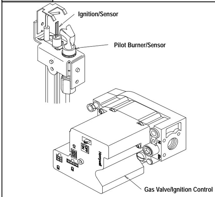
The system consists basically of only two (2) components. The Ignition System Control and the Pilot Hardware. The operate on Two (2) 24 volt power circuits received from the ST9160B Fan Timer/Furnace Control. One is the power supply to the ignitor, the second is to activate the ignition sequence.
