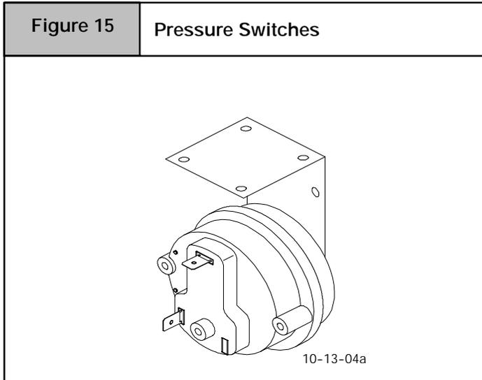
Under normal operating conditions, sufficient negative pressure will be created to close the pressure switch, and keep it closed to keep furnace operating. Under abnormal conditions, however, such as a restricted vent pipe, or a leak in one of the heat exchangers, sufficient negative pressure will not be created. This will result in the switch failing to close or failing to remain closed during furnace operation.
