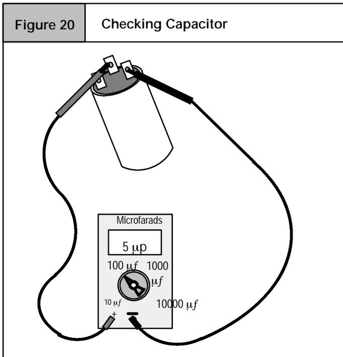
Capacitors are used for both the circulating (conditioned air) blower motor and the exhaust (combustion) blower. Before replacing one of these motors (assumed to be bad) the condition of its capacitor should be verified, since it, and not the motor, may be the source of the problem.
