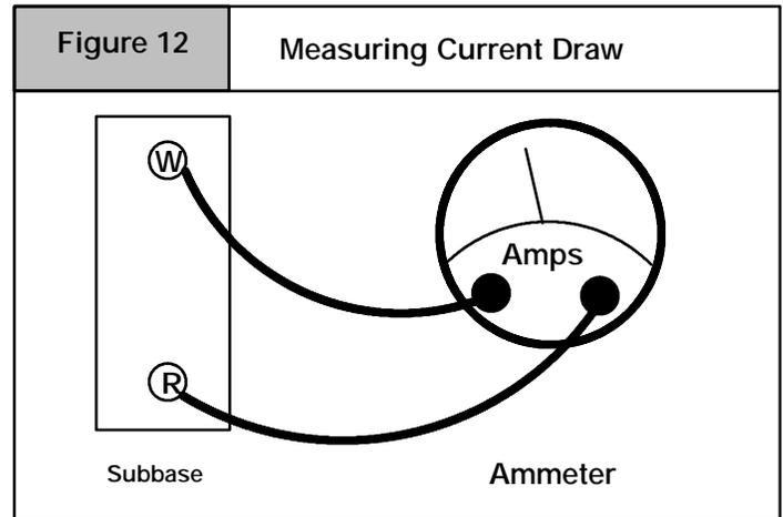
The best method to obtain the required setting for the heat anticipator, is to measure the actual current draw in the control circuit ("W") using a low range (0-2.0 Amps) Ammeter. (See **Figure 12**) After measuring the current draw, simply set the heat anticipator to match that value.
