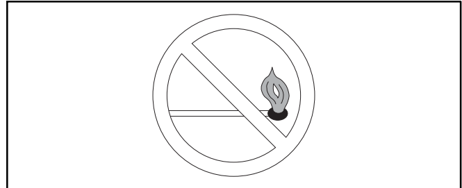
Figure 3 – Do Not Light Burner with Match
