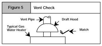
8. If improper venting is observed, the cause **MUST** be corrected.
