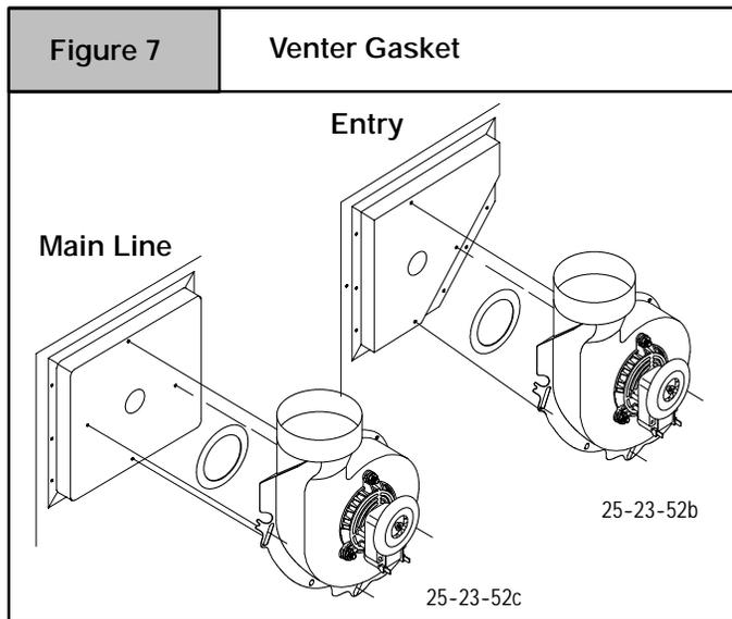
4. Replace venter gasket (part # 1013540, if needed) to venter assembly with adhesive in the same location as the old one.
