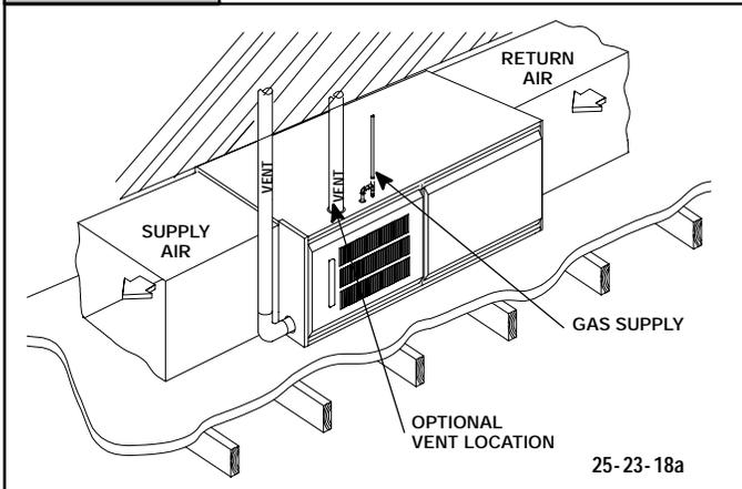
If the furnace is to be suspended from the floor joists in a basement or crawl space or the rafters in an attic, it is necessary to use steel pipe straps or an angle iron frame to attach the furnace. These straps should be attached to the furnace bottom side with sheet metal screws and to the rafters or joists with bolts. The preferred method is to use an angle iron frame bolted to the rafters or joists.
