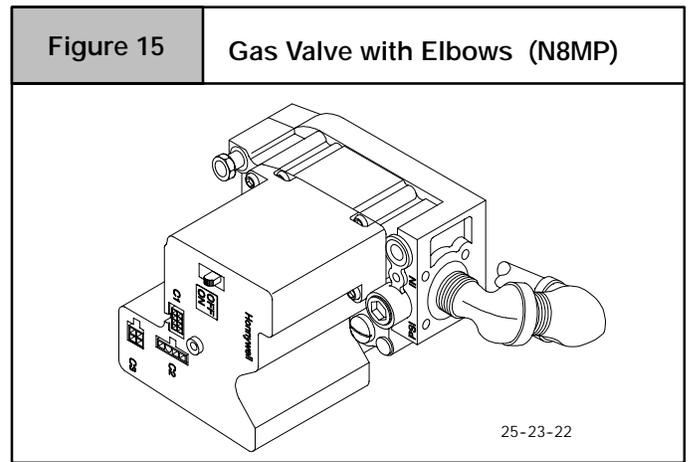
4. Gas supply line then can be run directly into opening of elbow.
