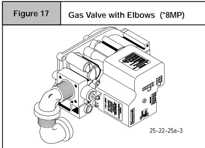
3. Turn assembly an additional  $\frac{1}{2}$  turn to position inlet near the top of the gas valve in line with gas opening on right side of furnace, see **Figure 18**.
