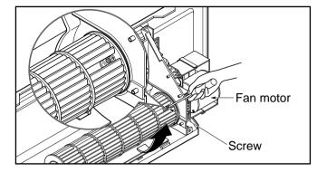
• Loosen the screw securing the mount motor.
