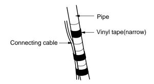
■ Bundle the piping and drain hose together by wrapping them with cloth tape over the range within which they fit into the rear piping housing section.
