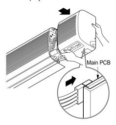
■ Refix the front right side panel to the original position with the two screws.
