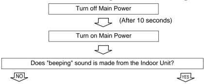
Check the voltage of power(About AC 220V/AC240V, 50Hz)
