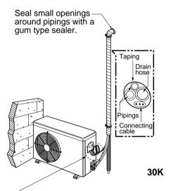
Trap is required to prevent water from entering into electrical parts.
