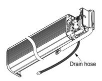
2. Insert the piping, drain hose and the connecting cable into the piping hole.
