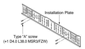
Measure the wall and mark the centerline. It is also important to use caution concerning the location of the installation plate-routing of the wiring to power outlets is through the walls typically.
