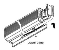
3. Remove the left side panel. (Remove the two screws.)
