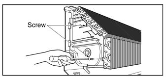
• Unhook the tab on the right inside of the chassis at the same time, slightly pull the evaporator toward you until the tab is clear of the slot.
