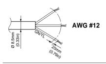
The connecting cable connected to the indoor and outdoor unit should be complied with the following specifications (UL and CSA recognized one).
