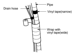
8. Reroute the pipings and the drain hose across the back of the chassis.
