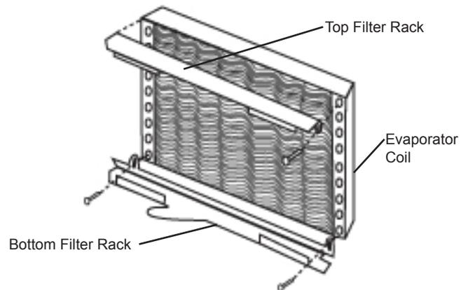
Fig. 1B - Filter Rack Installation (Straight Coil)
