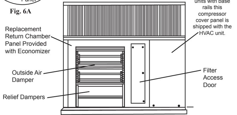
**Fig. 7 - Economizer Installed in HVAC Unit**
