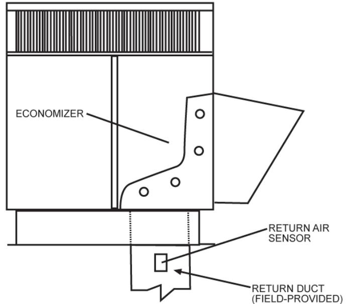
**Fig. 15 - Return Air Enthalpy Sensor Mounting Location**
