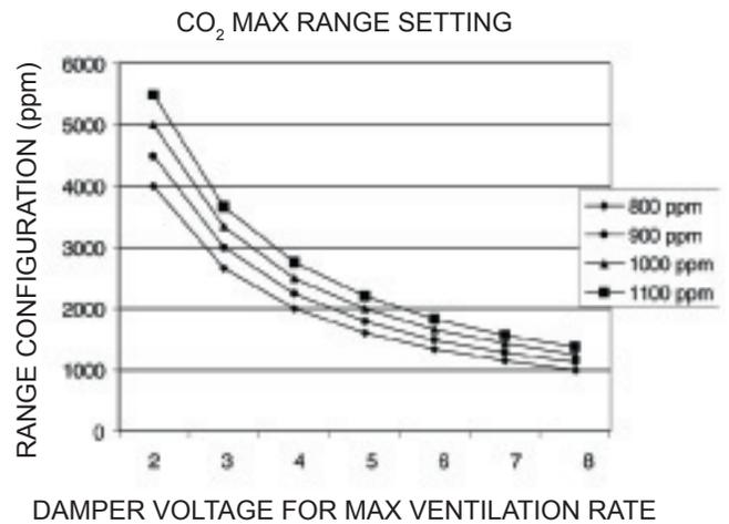
Fig. 18 - CO<sub>2</sub> Sensor Maximum Range Setting
