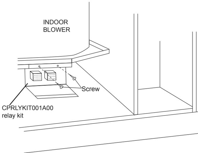
**Fig. 12 - Relay Kit Installation**
