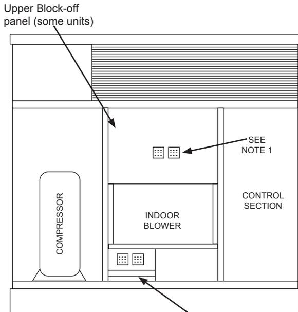
NOTE 1: Field provided relays can be mounted on upper block off panel, if applicable
