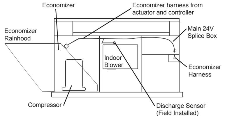
**Fig. 8 - Routing Harness Extension and Mounting SAT Sensor**
