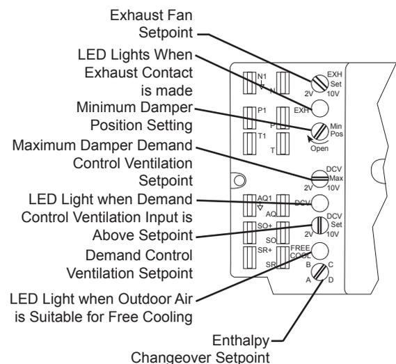
Fig. 13 - Economizer Controller Potentiometer LED Locations
