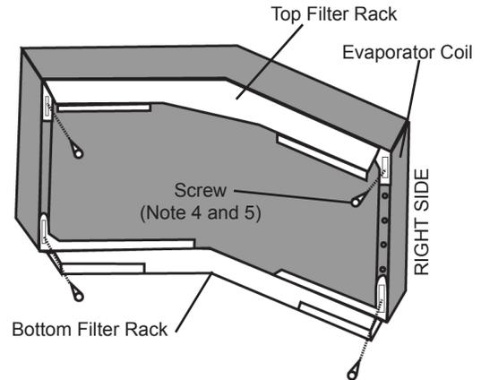
Fig. 1A - Filter Rack Installation (Bent Coil)
