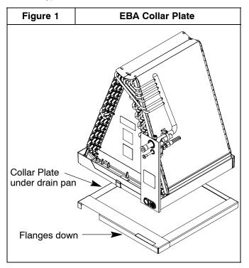
EBD Cased Coils are designed to fit furnaces and air handlers of the same width with no modifications. When an EBD Cased Coil is applied to a narrower or wider furnace or air handler, a field fabricated adapter is required. Refer to Figure 2 for examples of field fabricated adapters.
