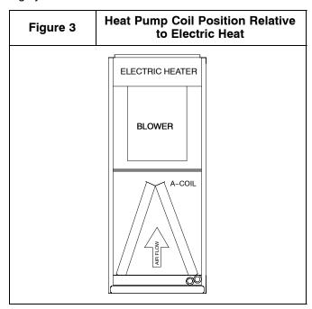
**NOTE:** When coil is installed with a Heat Pump in conjunction with a fossil fuel heating system, a Fossil Fuel Kit must be used. Refer to Product Specification literature for kit part number.
