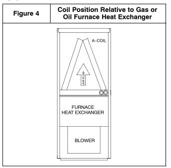
**NOTE:** On furnace installations where the coil is located in an unconditioned space, nuisance sweating may occur in the area around the cabinet to supply duct joint. Wrap the joint between the cabinet and the supply duct with a 6" wide piece of insulation with vapor barrier.
